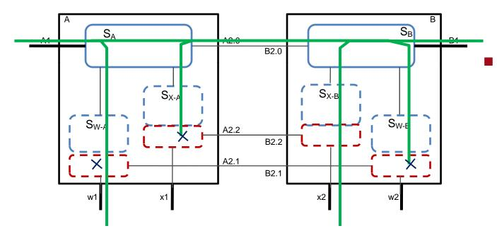
In a scenario where a service needs to span across multiple DRNIs, the service could be simply created on the logical port connected to the logical DRNI component.
