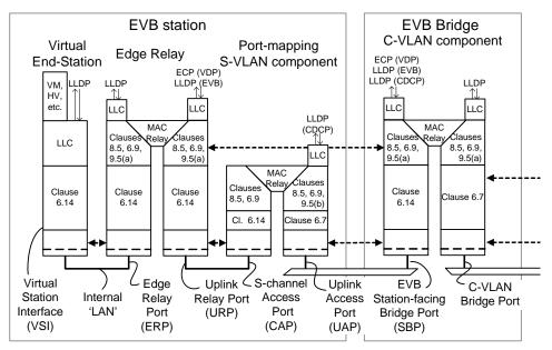
Figure 40-6—EVB architecture without S-channels including EVB station S-component
