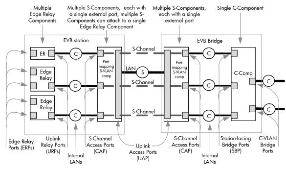
Figure 40-4—EVB components and internal LANs with S-channels
