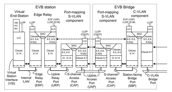
Figure 40-3—EVB archichtecture with S-channel
