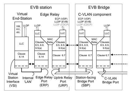
Figure 40-2—EVB architecture without S-channels
