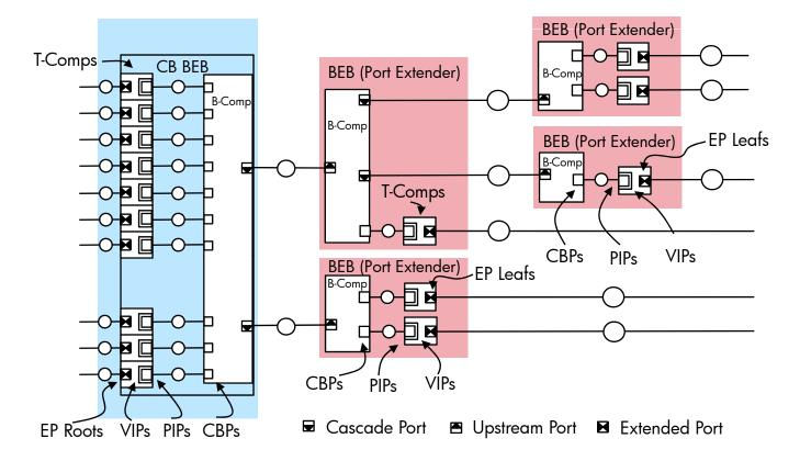
The Port Extender components of the Controlling Bridge along with the external Port Extenders make a complete PBBN which can support PBB-TE forwarding
