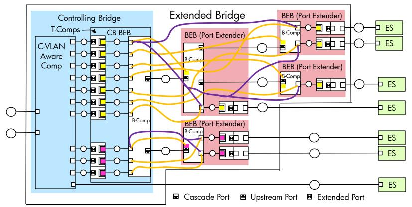
Tan lines in the diagram show the attachments of point-to-point TESIs
