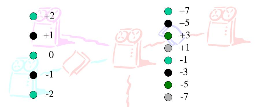
6dB co-set partitioning in 4DPAM-5 1000BASE-T (transmit 5 levels, but achieve noise immunity of 3 level signaling) 12dB co-set partitioning in a 4DPAM-8 10GBASE-T (transmit 8 levels, but achieve noise immunity of 2 level signaling)
