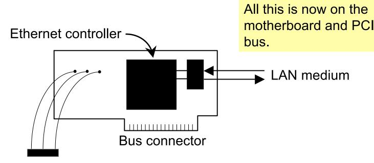
Cable and connector for auxiliary power and wake-up interrupt lines
