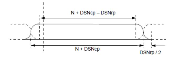
Figure 101–25—Cyclic prefix and windowing algorithm
