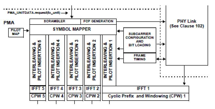
The DS symbol mapper takes one bit at a time across the PMA\_UNITDATA.request() and maps the bits into subcarriers, for all datacarrying subcarriers in a symbol, beginning at lowest frequency subcarrier, then moves to the next symbol. Since codewords can straddle frames, the first bit of the start of the first codeword following start of the next frame is sent in the current PHY Link (sounds complicated, but is straightforward).
