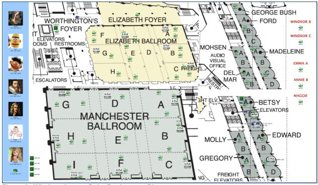
Figure 5. Wireless Access Point Deployment Plan
