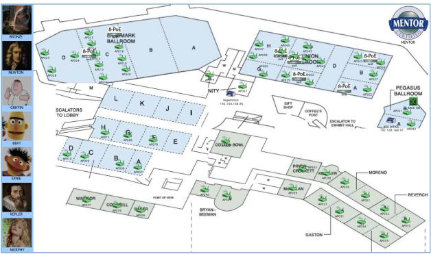
Figure 5. Wireless Access Point Deployment Plan
