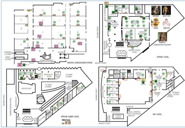
Figure 6. Wireless Access Point Deployment Plan
