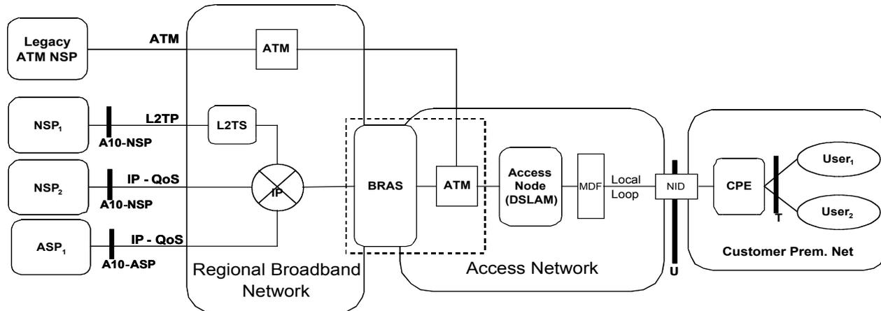
Figure 2- TR-059 High Level Architectural Reference Model
