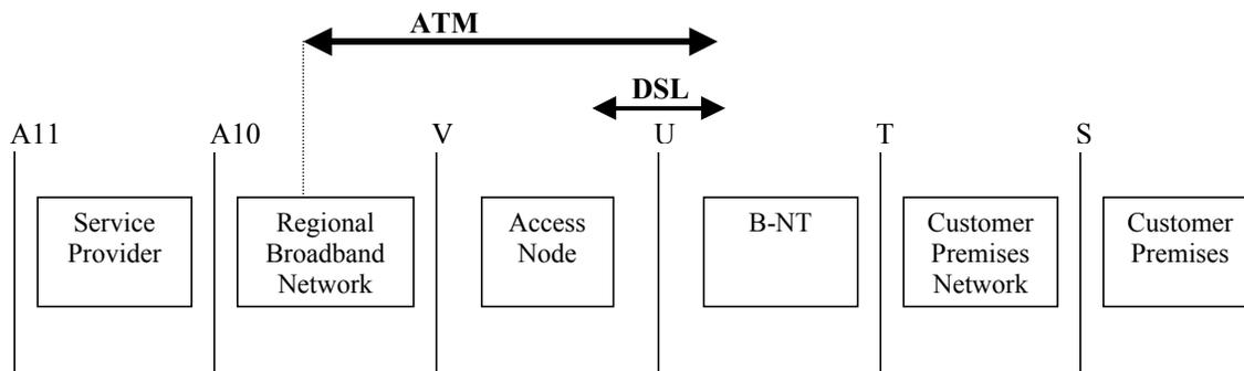
Figure 1 – TR-025 High Level Architectural Reference Model
