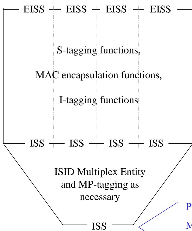
Customer data frames are constructed just as currently described in subclause 6.8 using the service-instance-with-encapsulated-ethernet tag (I-type).
