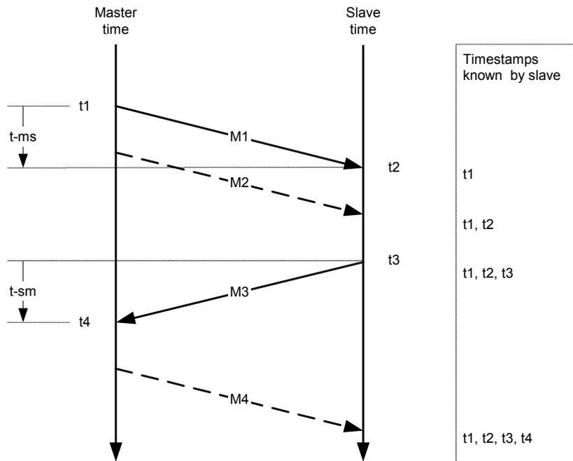
**Figure 3. Basic synchronization message exchange (taken from[9])**
