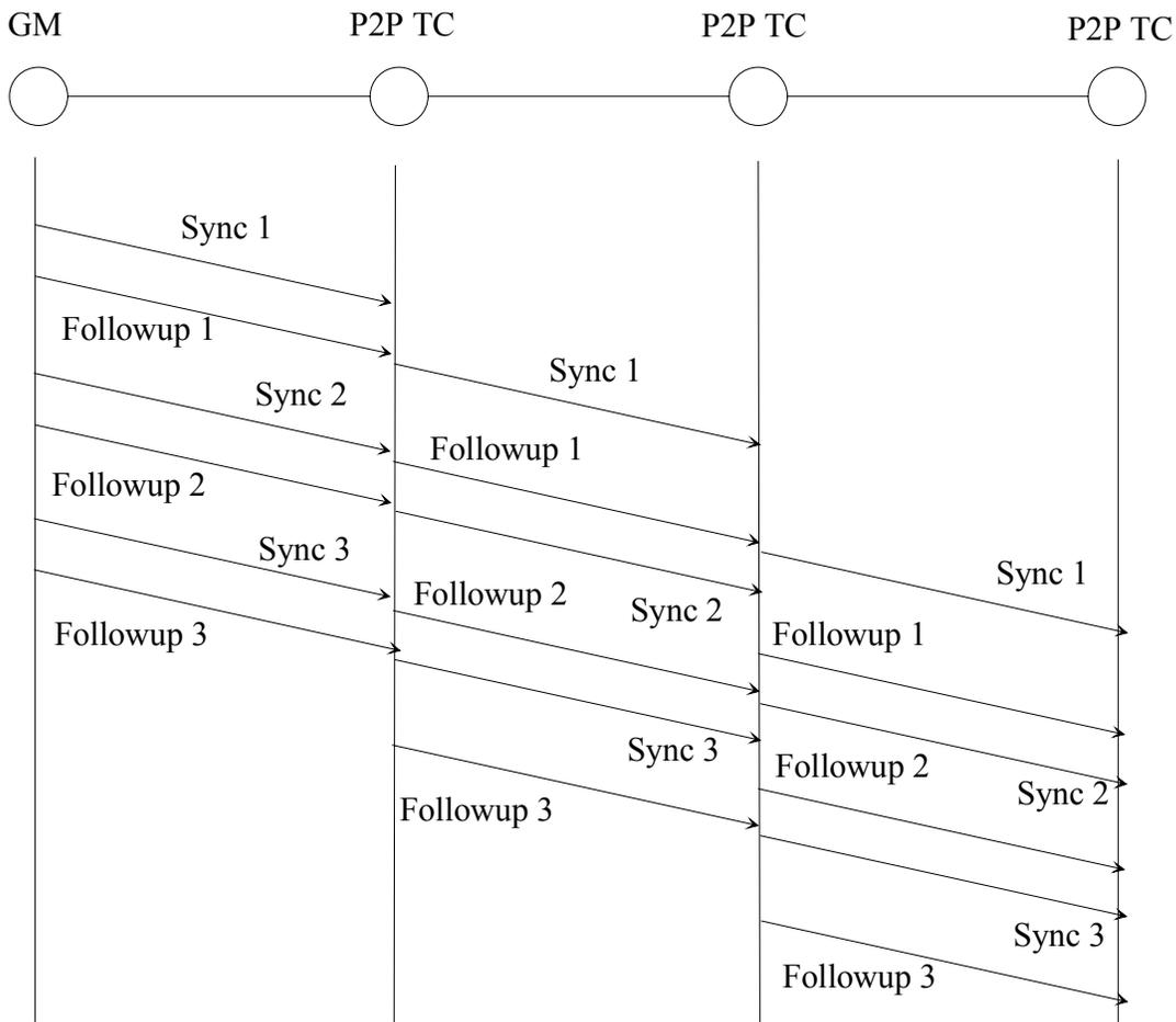
**Figure 6. Sync and Followup sent with Sync held at P2P TC until corresponding Followup arrives. Followup processing time and sync interval are of the same order. Sync processing time is much less than Followup processing time.**
