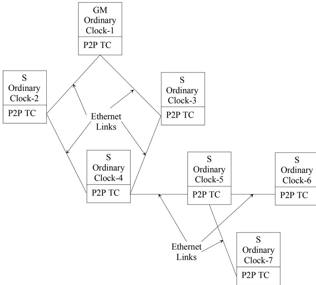
**Figure 2. Illustration of AVB clock hierarchy**
