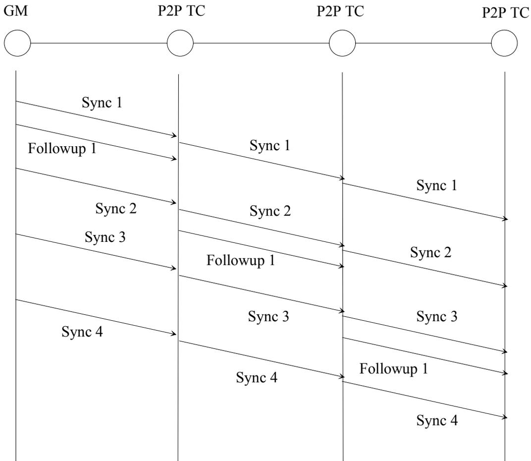
Note: The Followup messages corresponding to Sync2 and Sync3 are not shown to keep the diagram from being too cluttered.
