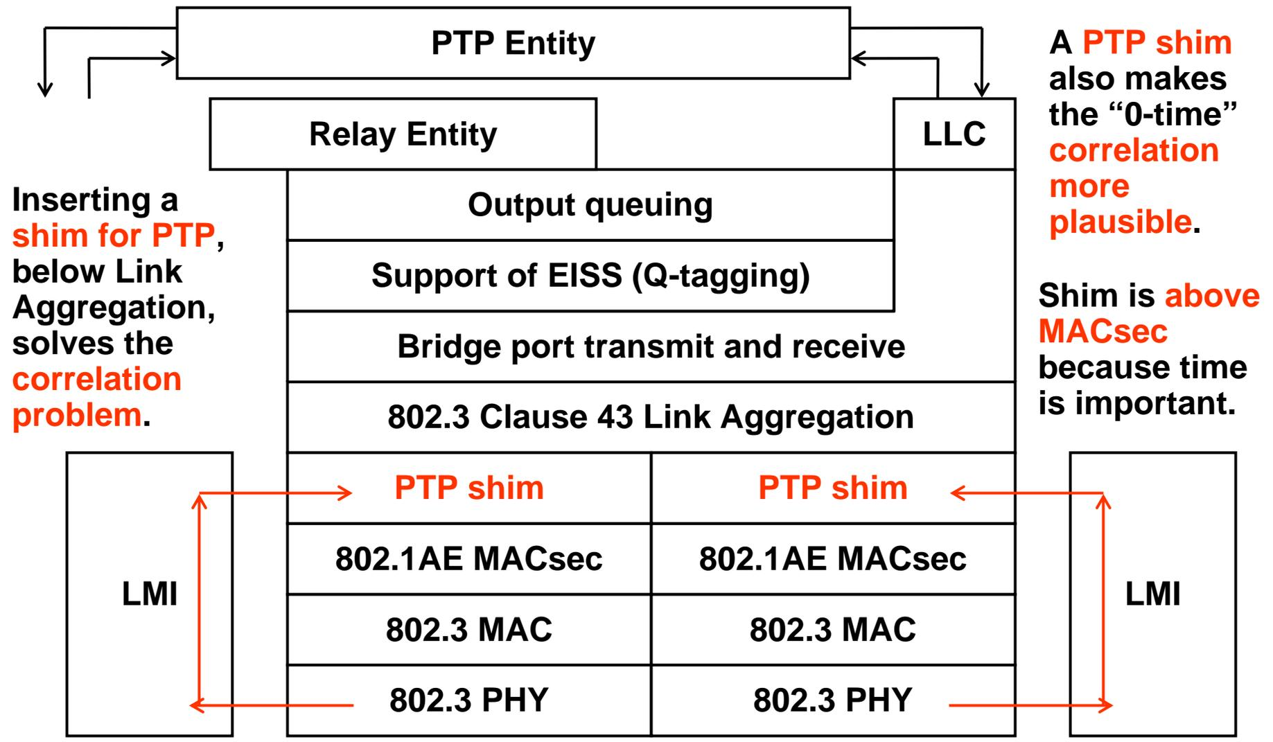
Inserting a **shim for PTP**, below Link Aggregation, solves the **correlation problem**.
