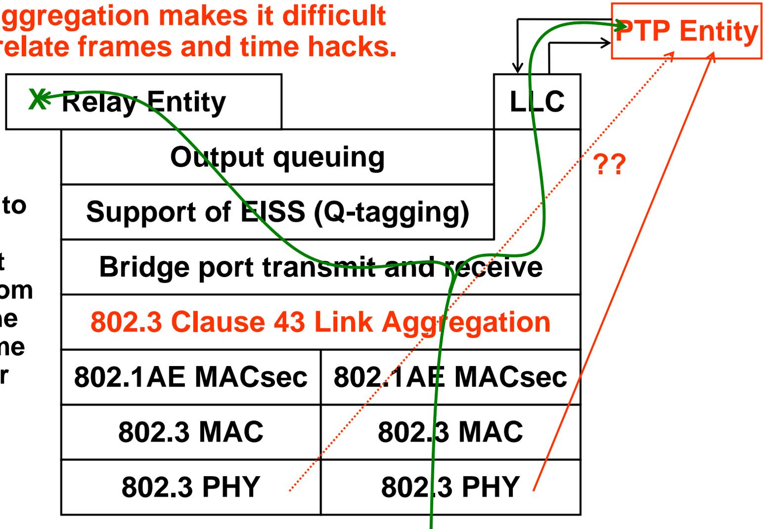
According to the model, you cannot **tell** to or from which of the links a frame was sent or received.
