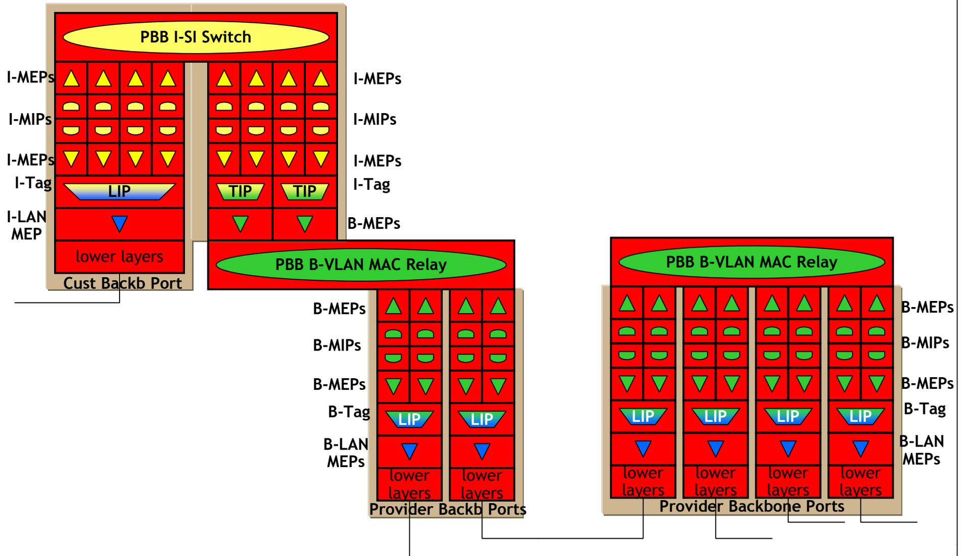
VIP: Virtual Instance Port, TIP: Trunk Instance Port, LIP: Link Instance Port
