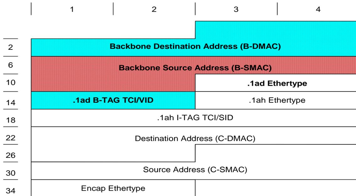
**Figure 3 802.1 PBB Header**
