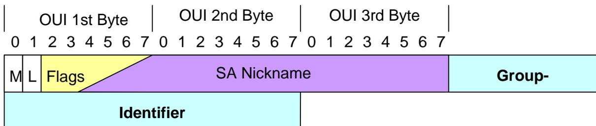
**Figure 5: Multicast B-DMAC Encoding**
