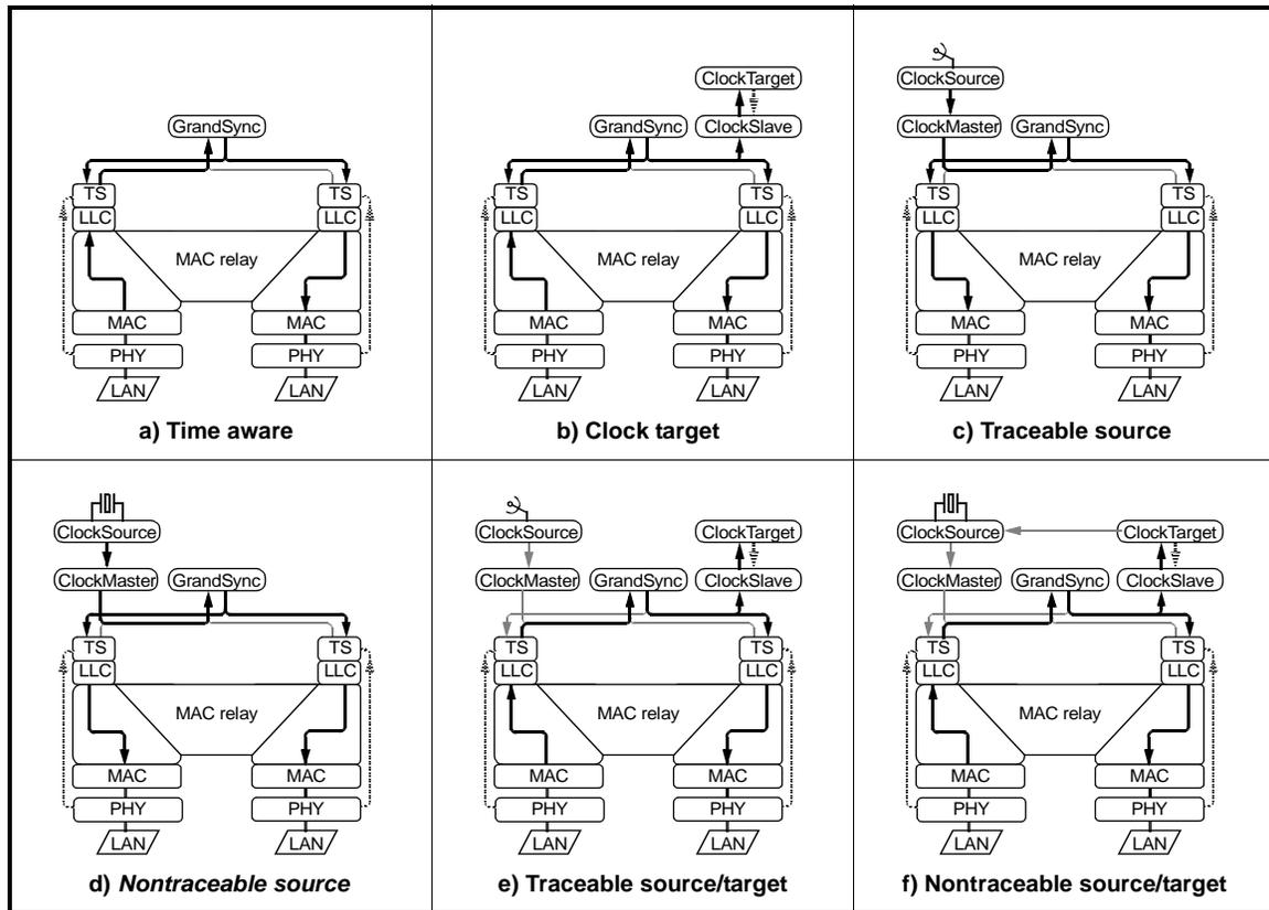
**Figure 5.15—Clock-attached time-aware bridge possibilities**
