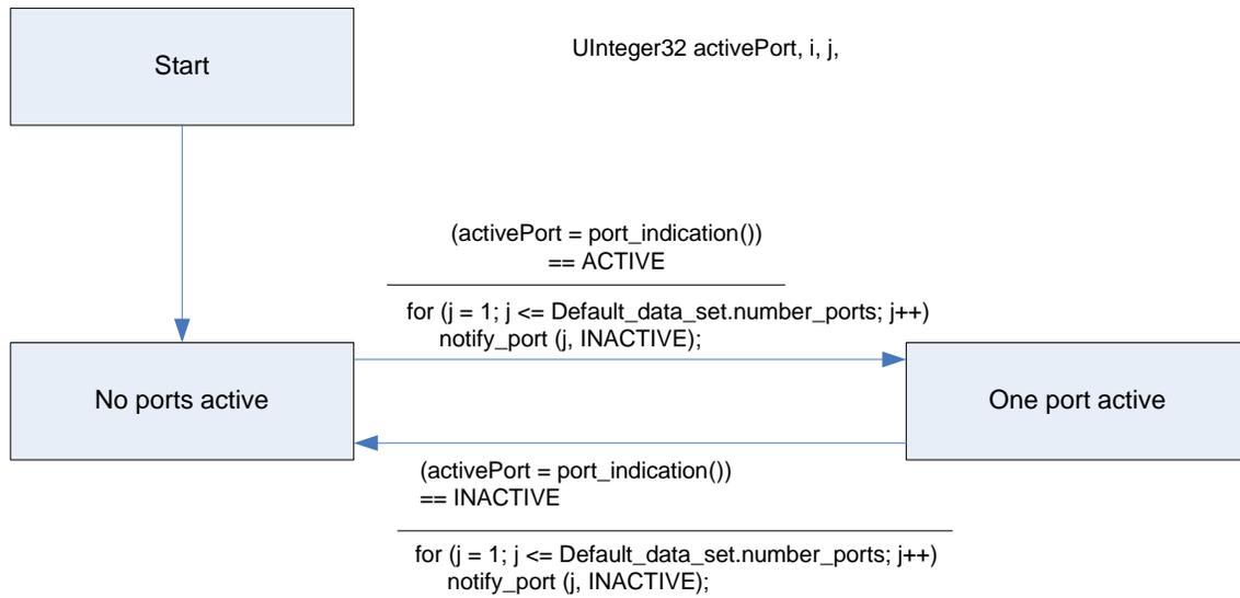
Figure 2-3. State machine, and corresponding C code, for a peer-to-peer transparent clock node
