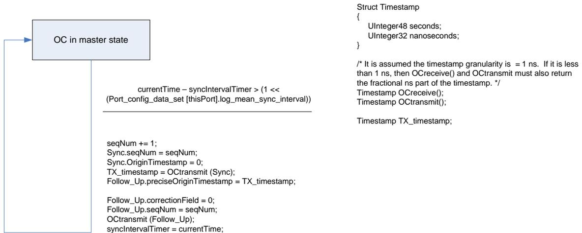
Figure 2-6. State machine, and corresponding C code, for sending of Sync and Follow\_Up by an ordinary clock
