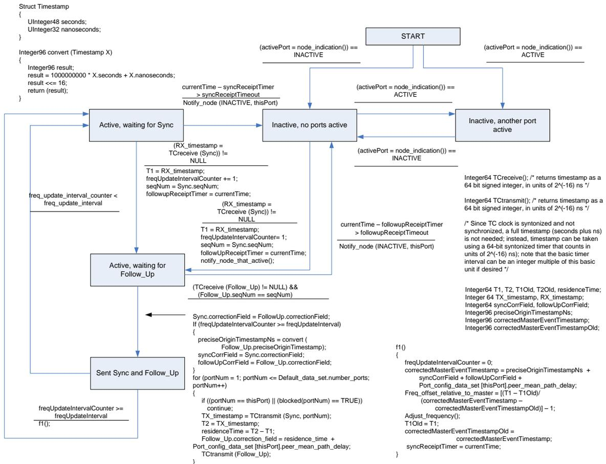
Figure 2-4. State machine, and corresponding C code, for receipt of Sync and Follow\_Up by a peer-to-peer transparent clock port
