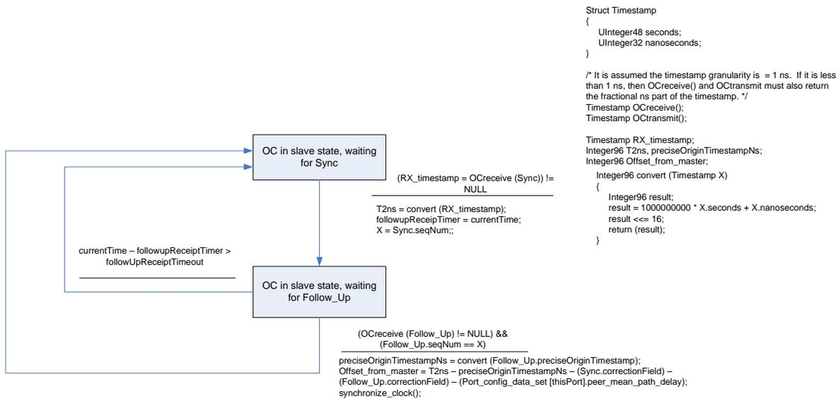
Figure 2-5. State machine, and corresponding C code, for receipt of Sync and Follow\_Up by an ordinary clock
