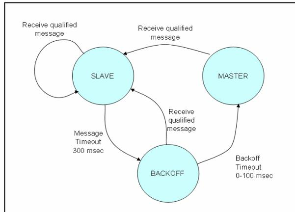
Figure 7-9. Clock Entity state diagram.
