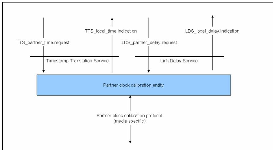
Figure 7-4. TTS and LDS interfaces.
