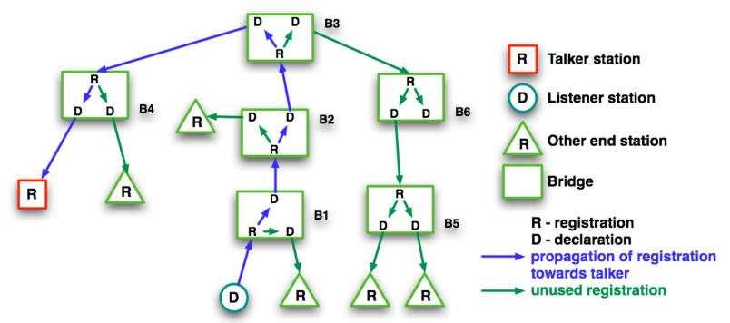
Reservation signaling triggers admission control operations in intermediate bridges. It also locks resources and updates filtering database if the admission control is successful.
