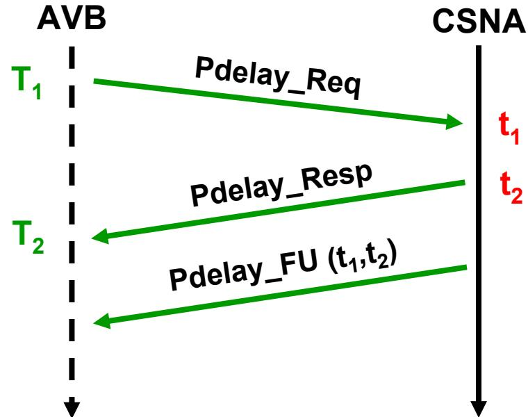
$$\text{LinkDelay}^* = ( (T_2 - T_1) - (t_2 - t_1) ) / 2$$
