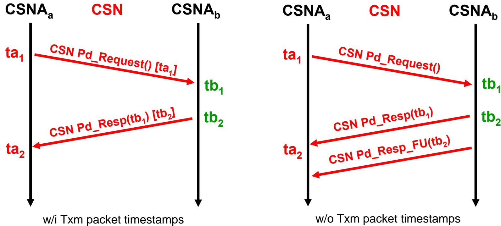
$$\text{CSN\_PropagationDelay} = \left( (ta_2 - ta_1) - (tb_2 - tb_1) \right) / 2$$
