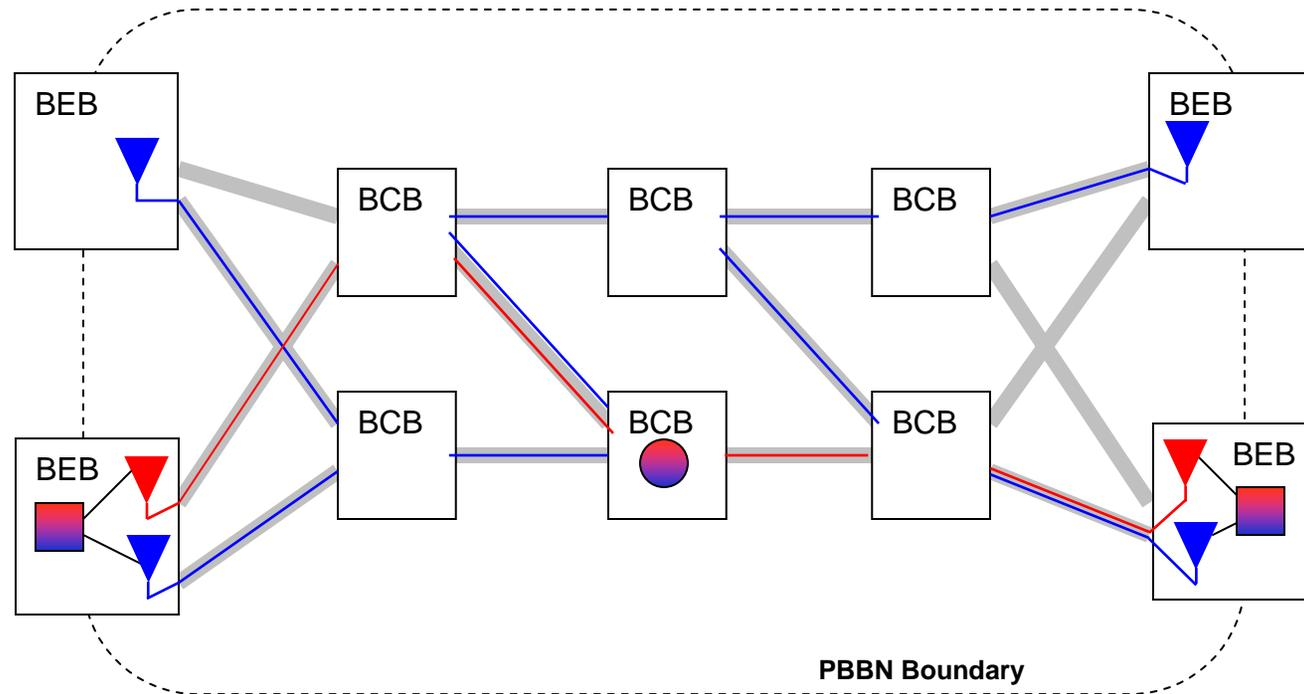
Scope of paths (CO) and BVLANS (CL) is defined by the PBBN boundary. CFM performed within this boundary is secure.
