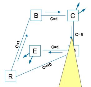
Σ of metrics of the "slow to converge" portion of the network needs to be greater than the rest of the loop, CD > DE+EB+BC
