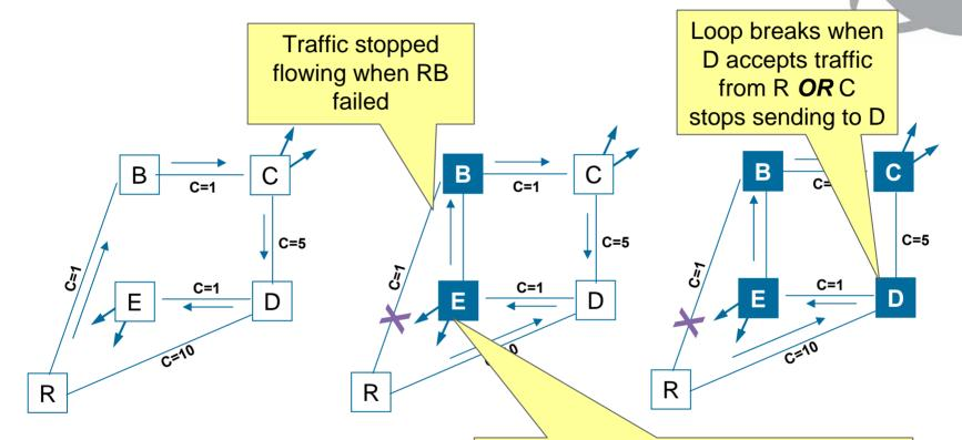
Traffic will only be trapped if loop RTT time > detection + notification + convergence time for B&E for both RB and EB link state changes Loop did not close until minimum of: detection time of RB failure
