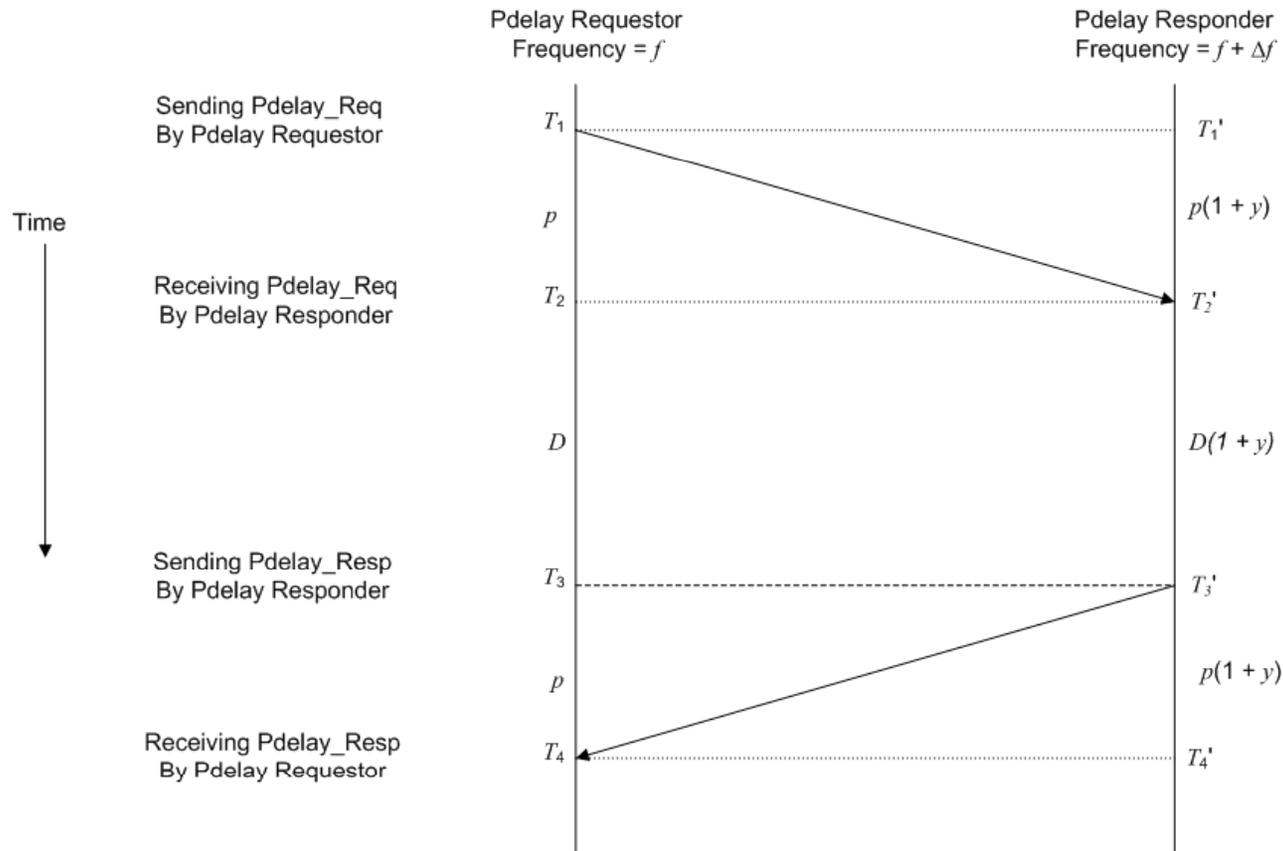
$p$  = propagation delay (assumed symmetric) relative to Pdelay Requestor
