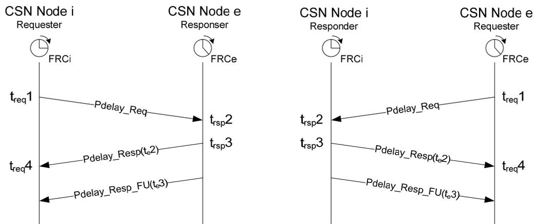
Figure 4: CSN Node to Node Path Delay Measurement without Network Clock reference
