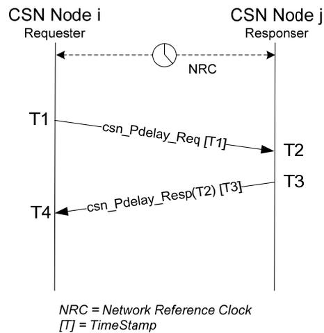
**Figure 5: CSN Node to Node Path Delay Measurement with Network Clock reference**
