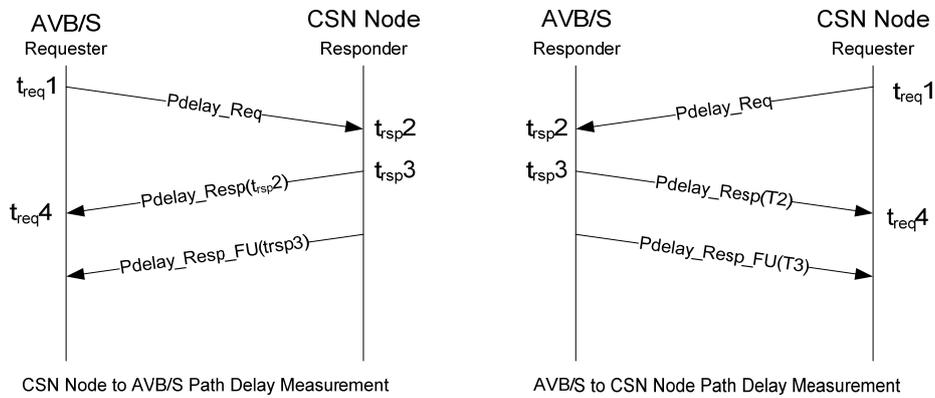
**Figure 3: Path Delay Measurements at the CSN Boundaries**
