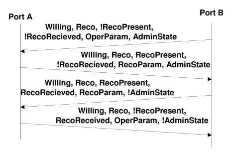
Two transfers in each direction required to transfer the parameters
