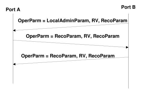
Two transfers in one direction and one transfer in the other direction required to transfer the parameters
