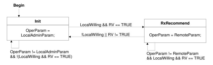
Note: RV can take on three values: TRUE, FALSE, and NULL. NULL indicates that the Recommendation TLV was not part of the last LLDP PDU received, or that no LLDP PDUs have been received.
