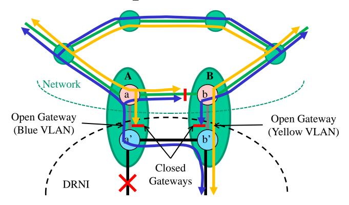
A failure of the DRNI link forces a change in the link selection for both VLANs. The gateway selection does not change, and therefore there is no change within the network.
