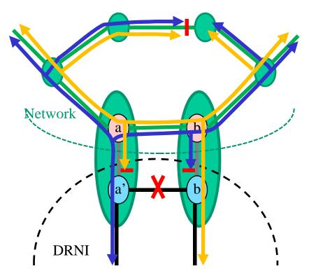
If the Intra-DAS Link failure is considered a failure in the DRNI, then the recovery method is to change the link selection for any VLANs using the Intra-DAS Link.
