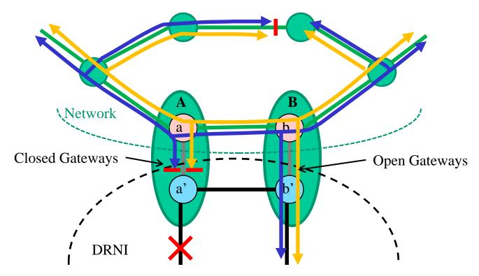
The network operator may choose to allow a change in the gateway selection as a result of the change in the link selection to make the data path more efficient. Changing the gateway reverses the direction of received DRNI frames on the path between A and B, however since the network link between A and B is in the active topology, the scope of the topology change is limited to the DRNI nodes and does not propagate to any other part of the network.
