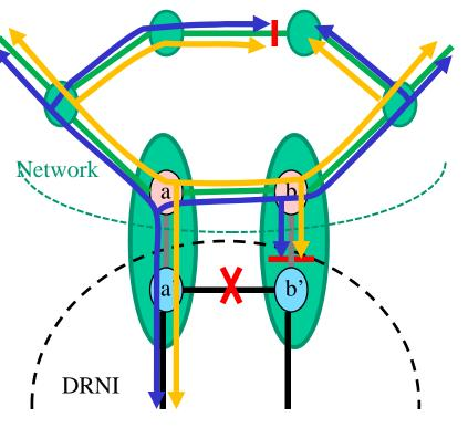
If the Intra-DAS Link failure is considered a failure in the network, then the recovery method is to change the gateway selection for any VLANs using the Intra-DAS Link. Changing the gateway reverses the direction of received DRNI frames on the path between A and B, which in this case contains the topology change to the DRNI nodes. 15
