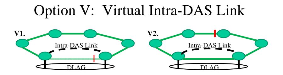
In this case the Intra-DAS Link is a virtual connection (a.k.a. tunnel) between the DRNI nodes.
