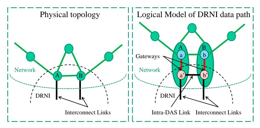
• The functionality of the Gateways, a', and b' are all in the Distributed Link Aggregation Sublayer.
