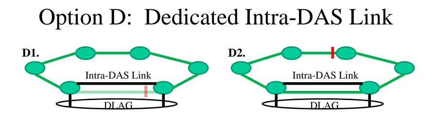
In this case the Intra-DAS Link is a direct physical link between the DRNI nodes dedicated to the Intra-DAS Link function.
