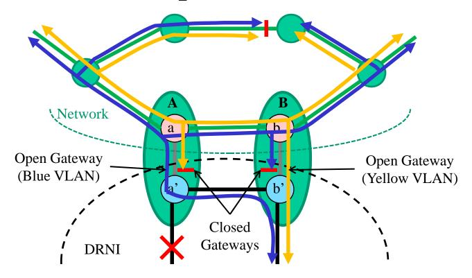
DRNI link failure forces a link selection change in the selected link. Neither the failure itself nor the resulting link selection change force a gateway selection change, however the resultant data path of the Blue VLAN is inefficient.
