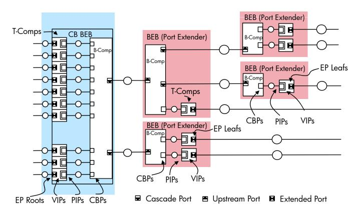
The Port Extender components of the Controlling Bridge along with the external Port Extenders make a complete PBBN which can support PBB-TE forwarding
