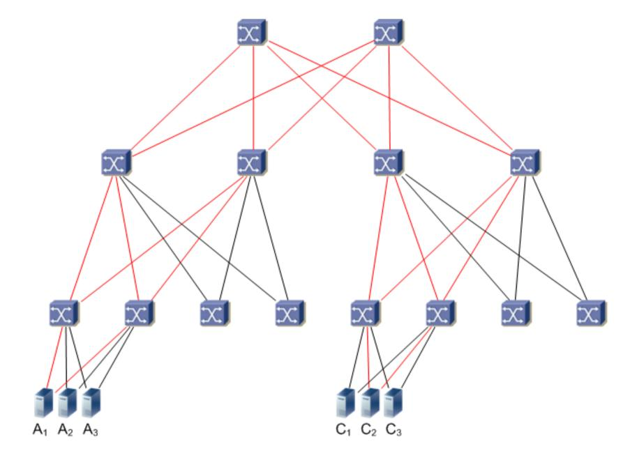
ECMP load spreading utilizes all links on equal cost paths for unicast traffic.
