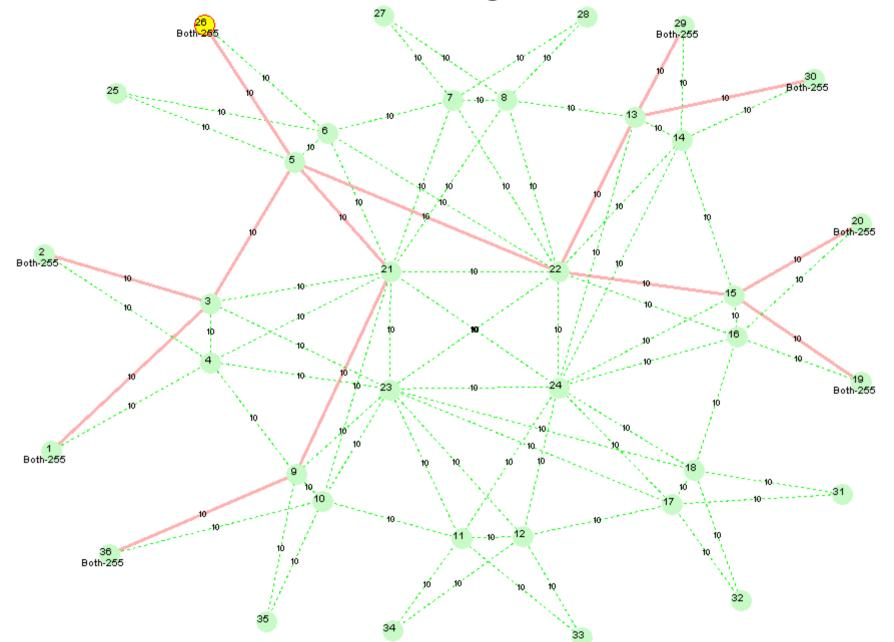
Multicast selects links from one equal cost tree using ECT tie-breaker.
