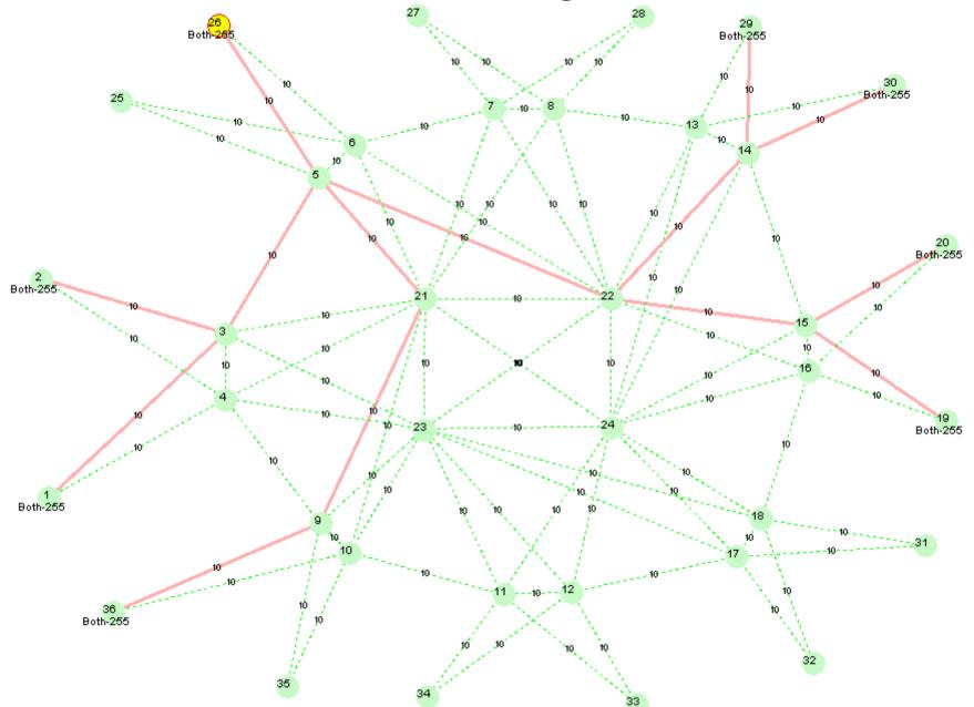
Multicast load spreading selects links from all equal cost paths using a hash function (in this case FNV).
