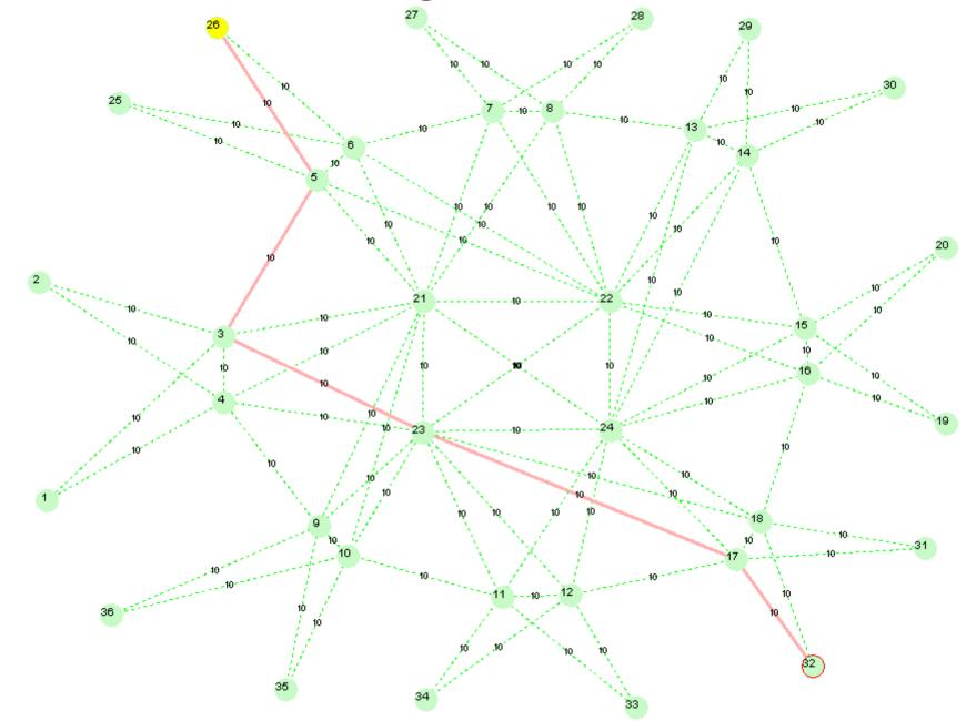
SPB selects a single path using an ECT tie-breaking function.
