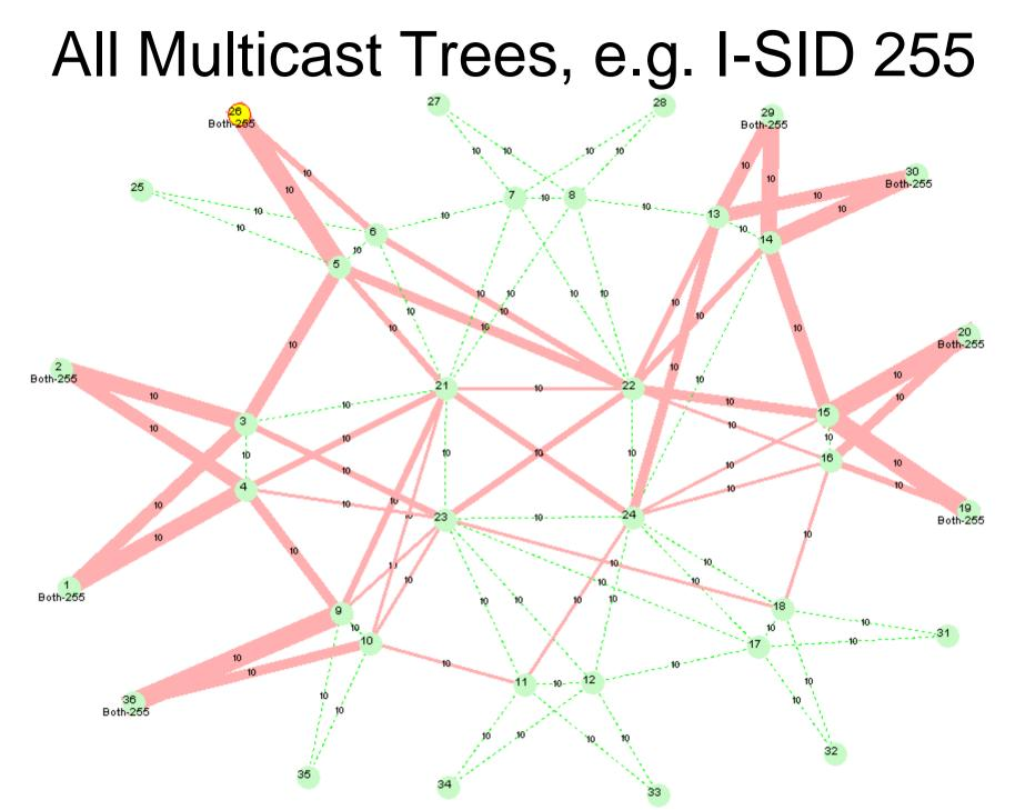
Multicast load spreading selects links from all equal cost paths using a hash function (in this case FNV). Different trees are selected for each root by including root MAC address in hash.
