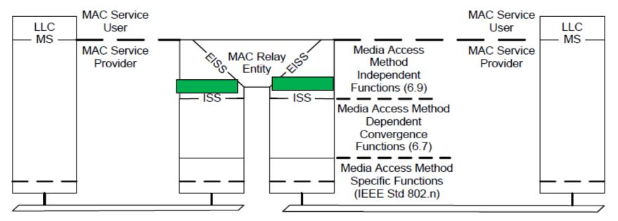
NOTE—The notation "IEEE Std 802.n" in this figure indicates that the specifications for these functions can be found in the relevant standard for the media access method concerned; for example, n would be 3 (IEEE Std 802.3) in the case of Ethernet.
