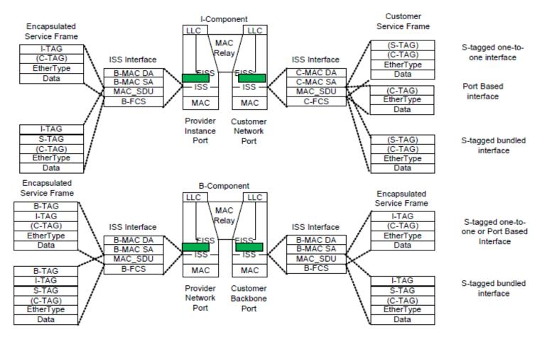
Figure 25-6—Encapsulated service frames at ISS
