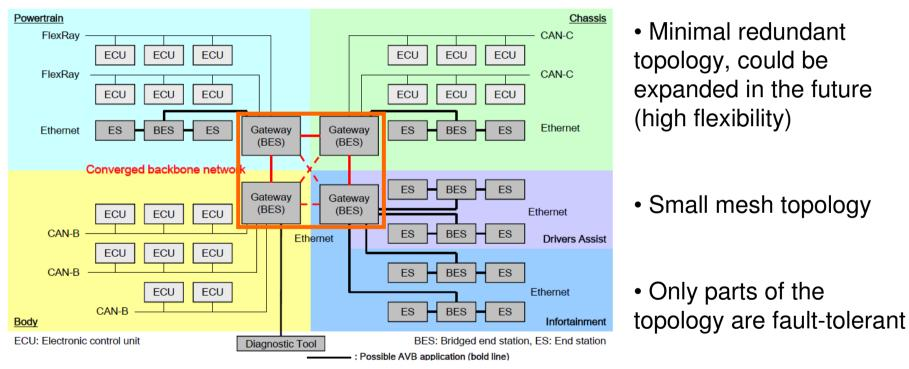
• Mesh keeps total hop count low, but introduces strong requirements on redundancy control protocol in fault-tolerant segments when combined with demanding timing requirements
