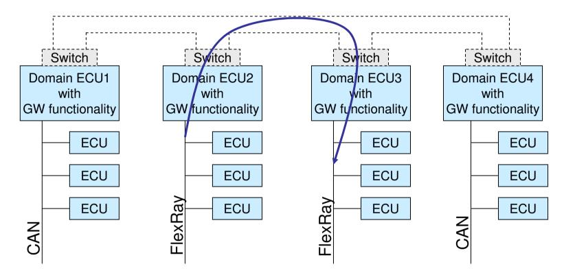
Transmission of FlexRay-Frames between FlexRay-Clusters where the timing information (slot/cycle count) of a FR-message is required
