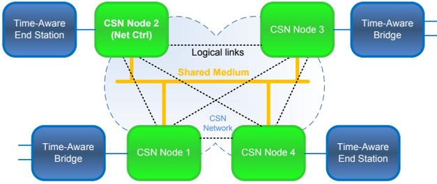
Fig. 5: Example of CSN Backbone in an AVB LAN
