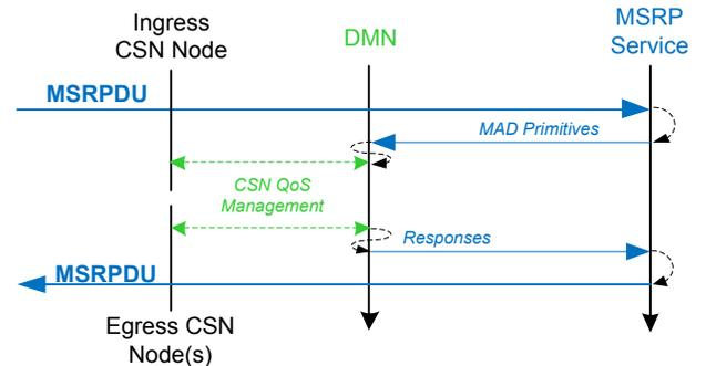
Fig. 7: MSR PDU Flow over CSN
