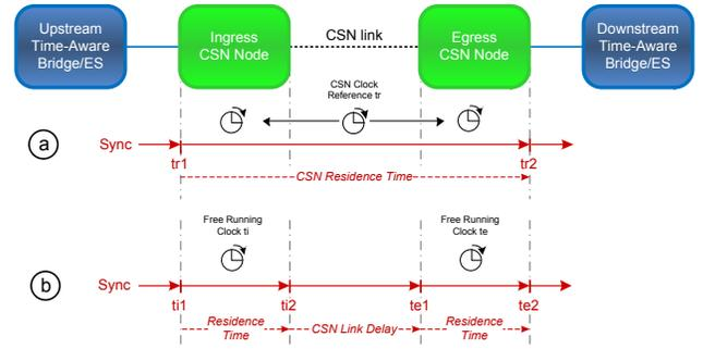
Fig. 6: IEEE 802.1AS Sync Message Propagation over CSN
