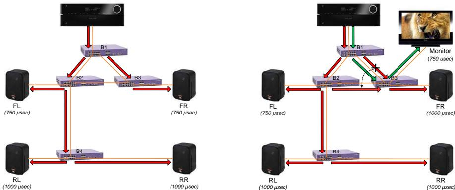
In this example the FL & FR speakers inform the network they can accept latency up to 1000 usec and still play in sync with the RL & RR speakers. This allows the network to reconfigure the audio path to the FR speaker when the video reservation is established. The RL & RR speakers still require the latency guarantees provided by MSRPv0.
