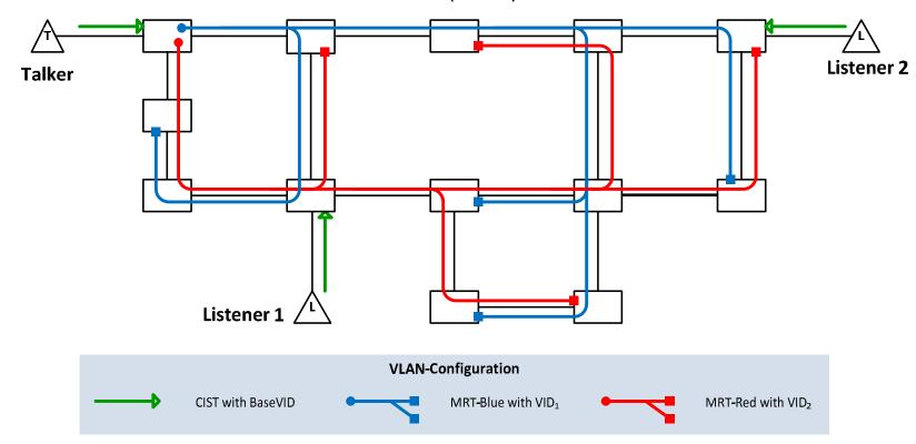
Assumption: pre-installed Maximal Redundant Trees (MRT)
