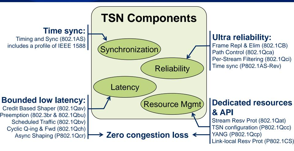
Guaranteed data transport with bounded low latency, low delay variation, and extremely low loss
