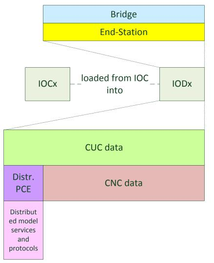
IOD loaded by IOC, with CUC and CNC data. CNC data is persistent stored in IOD.
