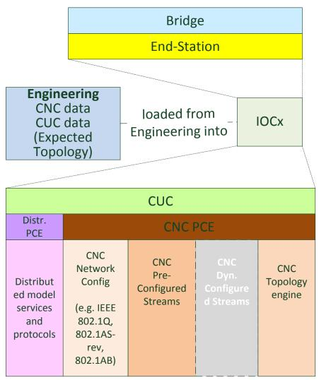
IOC loaded by engineering, with CUC, CNC and if required by customer with expected topology data. Engineering is afterward removed from the system.
