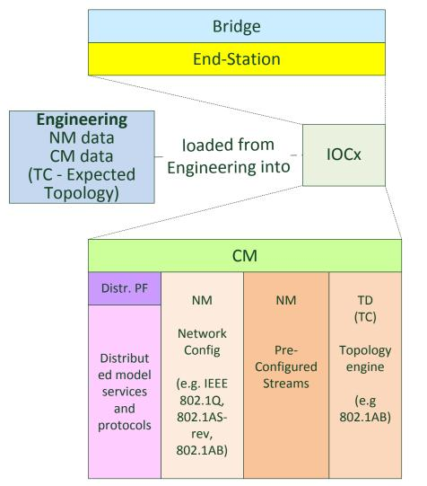
IOC loaded by engineering, with NM, CM and if required by customer with expected topology data. Engineering is afterwards removed from the system.
