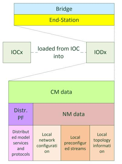
IOD loaded by IOC, with NM and CM data. NM data is persistent stored in IOD. NM data configures the local bridge and end-station. CM data is used for stream establishment and may be dynamically changed by the IOC over time. Topology information is provided for TD and offers checking of expected neighbors, too.
