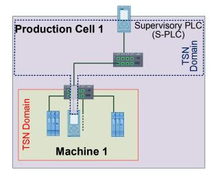
Figure 52 gives an example of M2M communication to a supervisory PLC.
