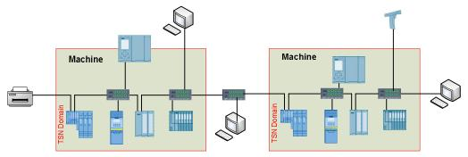
Figure 57 – pass-through two machines
