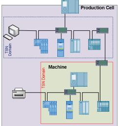
Figure 56 – pass-through one machine and production cell
