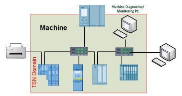
Figure 58 – machine with diagnostics / monitoring PC
