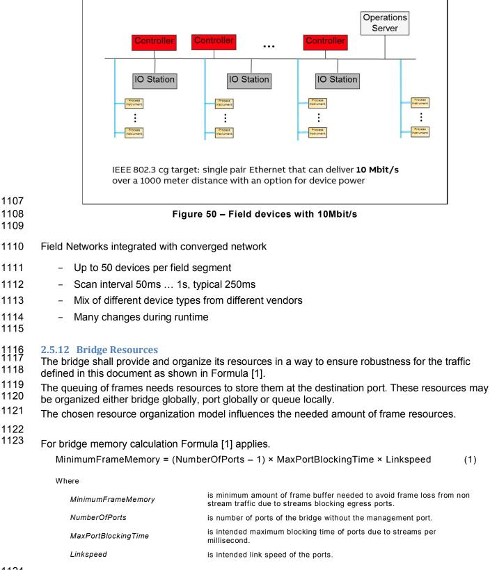
Formula [1] assumes that all ports use the same link speed and a bridge global frame resource management. Table 13, Table 14, Table 15, and Table 16 shows the resulting values for different link speeds and fully utilized links. 1128 The traffic from the management port to the network needs a fair share of the bridge resources to
