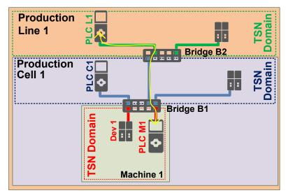
Figure 5 – Three TSN domains connected by Bridges
