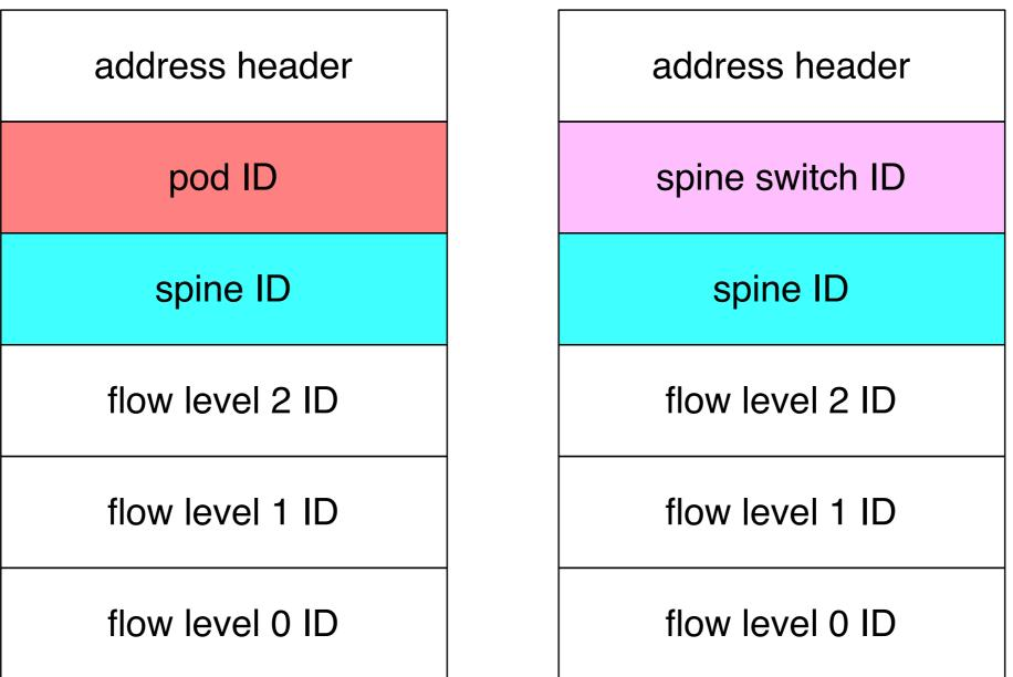
Note 1: server and rack switch format is similar to data-plane address Note 2: each address format needs to be distinct (in header or otherwise)
