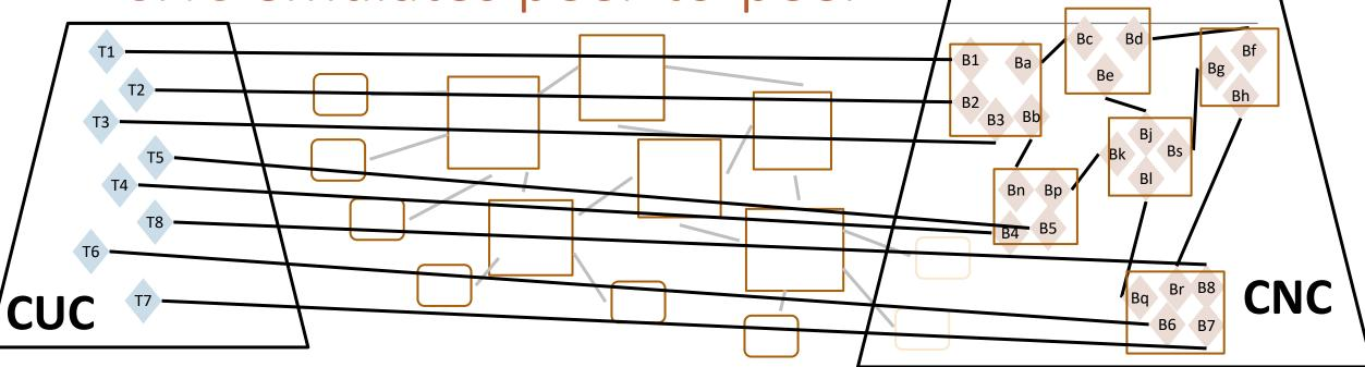
**CUC** controls Talkers, **CNC** controls Bridges.
