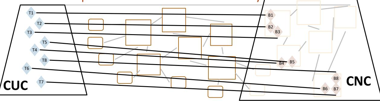
**CUC** controls Talkers, **CNC** controls Bridges.
