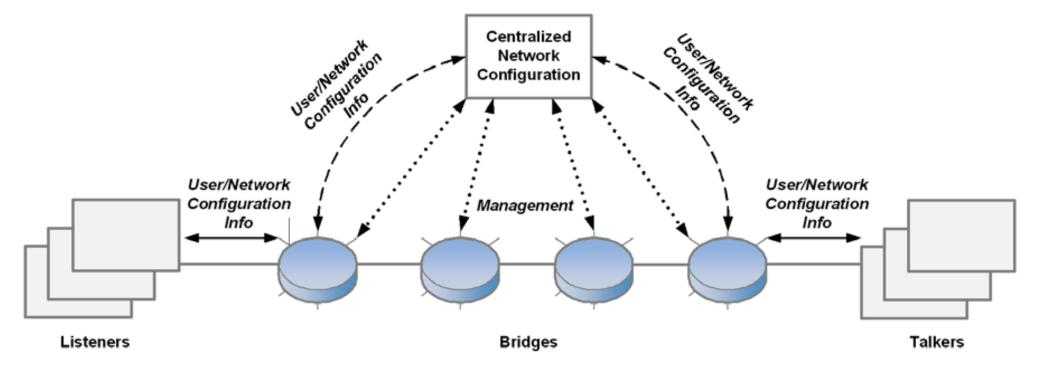
Figure 46-2 — Centralized Network / Distributed User Model
