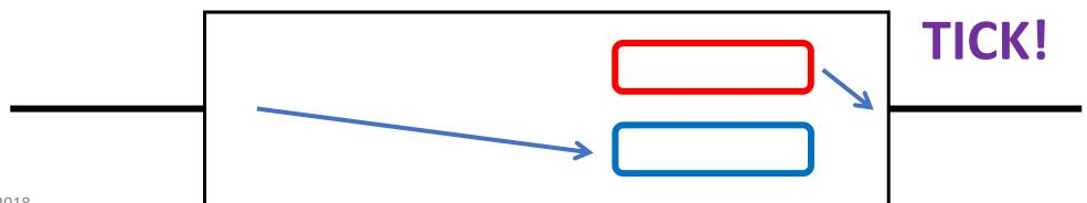
• Two-buffer version: Two buffers per port. Input and output buffers swap at the same moment, once every cycle, period  $T_c$ . Small guard band to allow for transit and forwarding time. All relay nodes are synchronized and swap buffers at the same moment. Cycle time  $T_c$  > transit time + forwarding time + clock inaccuracy + max data transmit time.
