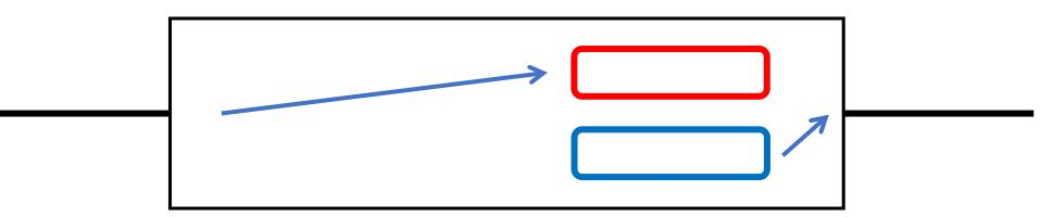
• Two-buffer version: Two buffers per port. Input and output buffers swap at the same moment, once every cycle, period  $T_c$ . Small guard band to allow for transit and forwarding time. All relay nodes are synchronized and swap buffers at the same moment. Cycle time  $T_c$  > transit time + forwarding time + clock inaccuracy + max data transmit time.
