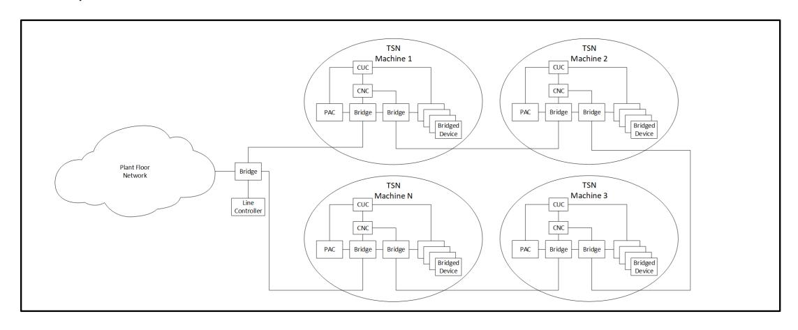
TSN Domain: A set of stations (end stations and/or Bridges), their Ports, and the attached individual LAN's that transmit Time—Sensitive Streams using TSN standards which include Transmission Selection Algorithms, Preemption, Time Synchronization and Enhancements for Scheduled Traffic and that share a common management mechanism (or "policy engine").
