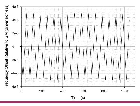
Case 1, PTP Instance (node) 50 Filtered phase offset relative to GM Clock Model: Triangular wave phase and freqeuncy error variation, with zero phase offset of this variation at each node) Residence Time: 1 ms, 4 ms, 10 ms with equal probability (chosen independently for each Sync message)
