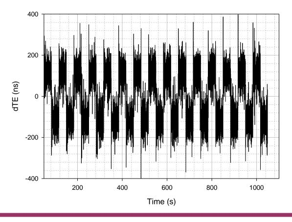
Case 1, PTP Instance (node) 90 Filtered phase offset relative to GM Clock Model: Triangular wave phase and freqeuncy error variation, with zero phase offset of this variation at each node) Residence Time: 1 ms, 4 ms, 10 ms with equal probability (chosen independently for each Sync message) First 50 s omitted to eliminate any startup transient
