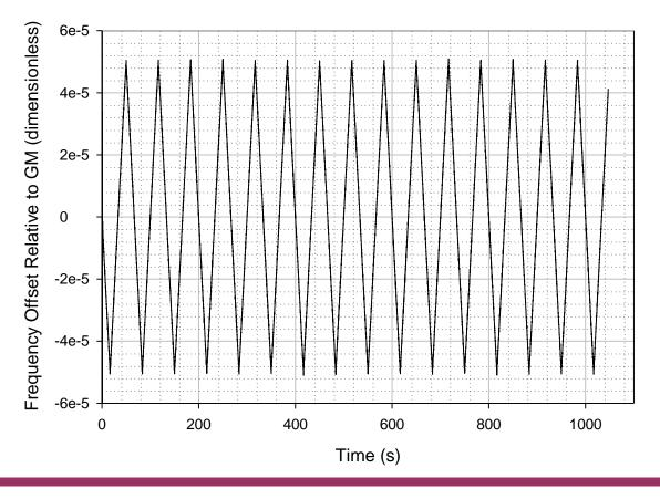
Case 1, PTP Instance (node) 70 Filtered phase offset relative to GM Clock Model: Triangular wave phase and freqeuncy error variation, with zero phase offset of this variation at each node) Residence Time: 1 ms, 4 ms, 10 ms with equal probability (chosen independently for each Sync message) First 50 s omitted to eliminate any startup transient
