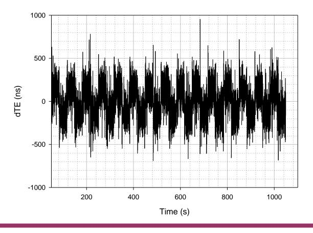
Case 1, PTP Instance (node) 100 Filtered phase offset relative to GM Clock Model: Triangular wave phase and freqeuncy error variation, with zero phase offset of this variation at each node) Residence Time: 1 ms, 4 ms, 10 ms with equal probability (chosen independently for each Sync message) First 50 s omitted to eliminate any startup transient
