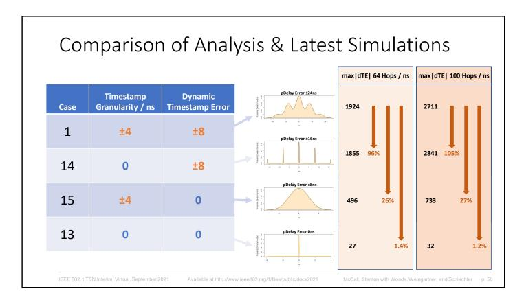
Note that the simulation removed the effects of Timestamp Granularity and Dynamicstamp Error from both pDelay and Residence Time.
