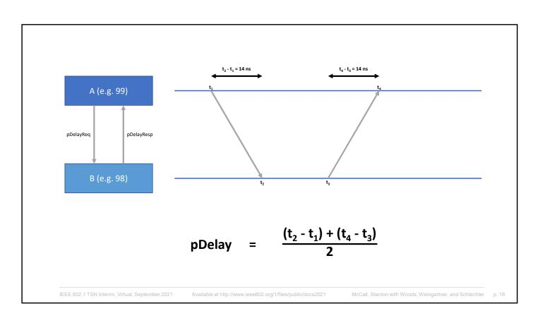
This is the idealised view...the Platonic ideal of how pDelay is measured.
