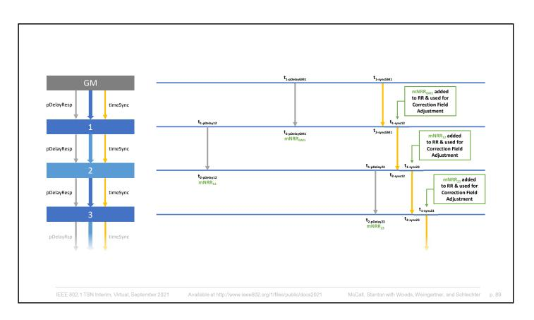
NRR is measured at last pDelay message (mNRR)...but added to Rate Ratio at end of Residence Time (Time Sync message TX). This means that the amount of adjustment to Rate Ratio (i.e. NRR) is effectively measured at mNRR.
