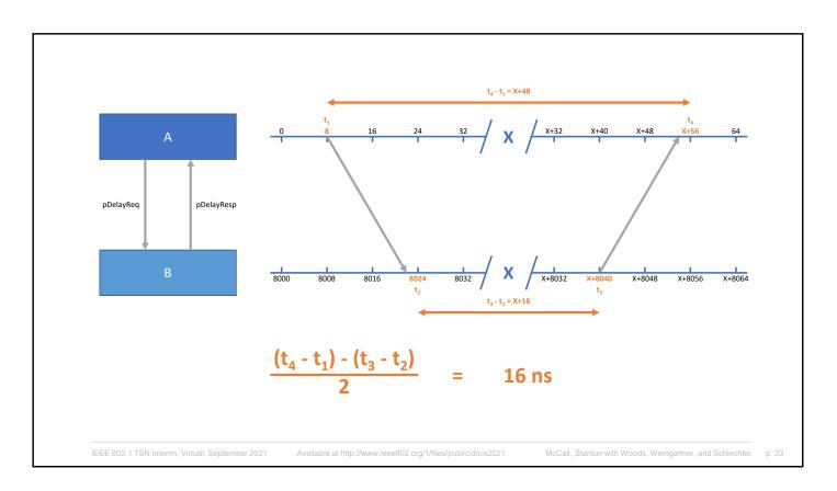
Firstly, there is a relatively large amount of time between the left and right ends of the timeline due to the fact that pDelay Response Time is much longer than pDelay...a fact I previously ignored.
