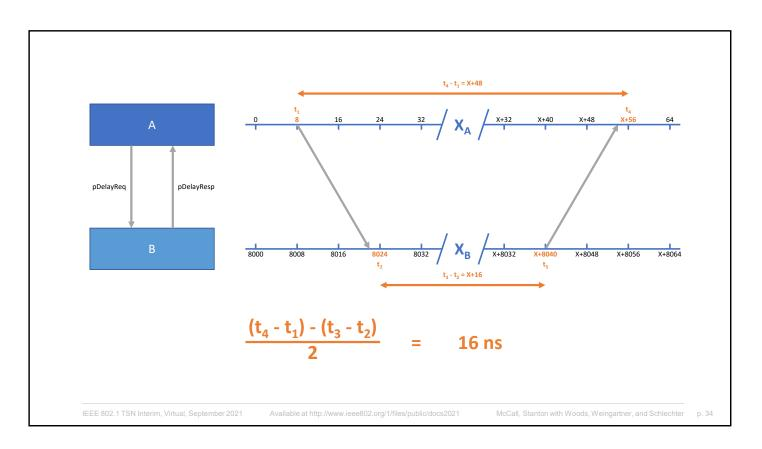
And secondly, that relatively long period of time is measured by two free running local clocks. Running at different speeds...and drifting slightly relative to each other.
