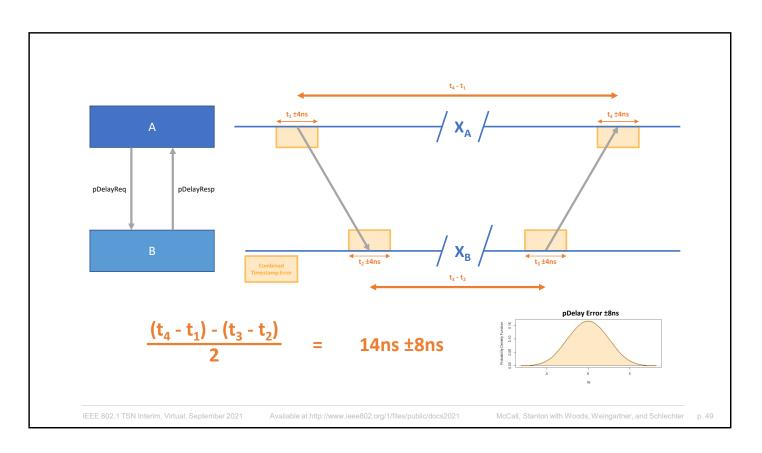
Case 15 in 60802-garner-new-simulation-results-new-freq-stab-model-0421-v02.pdf
