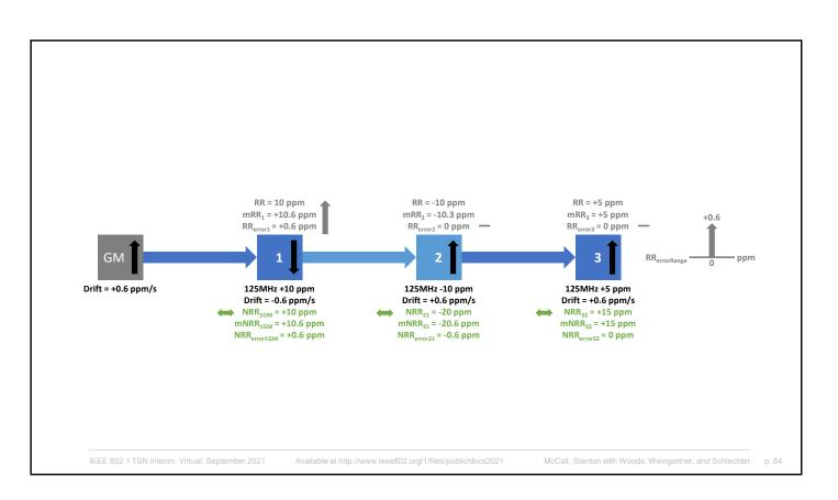
Adding Clock Drift to the GM is very different because it affects the Rate Ratio Error at every single downstream device.
