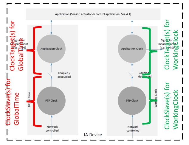
Figure 7 - Clock usage principles
