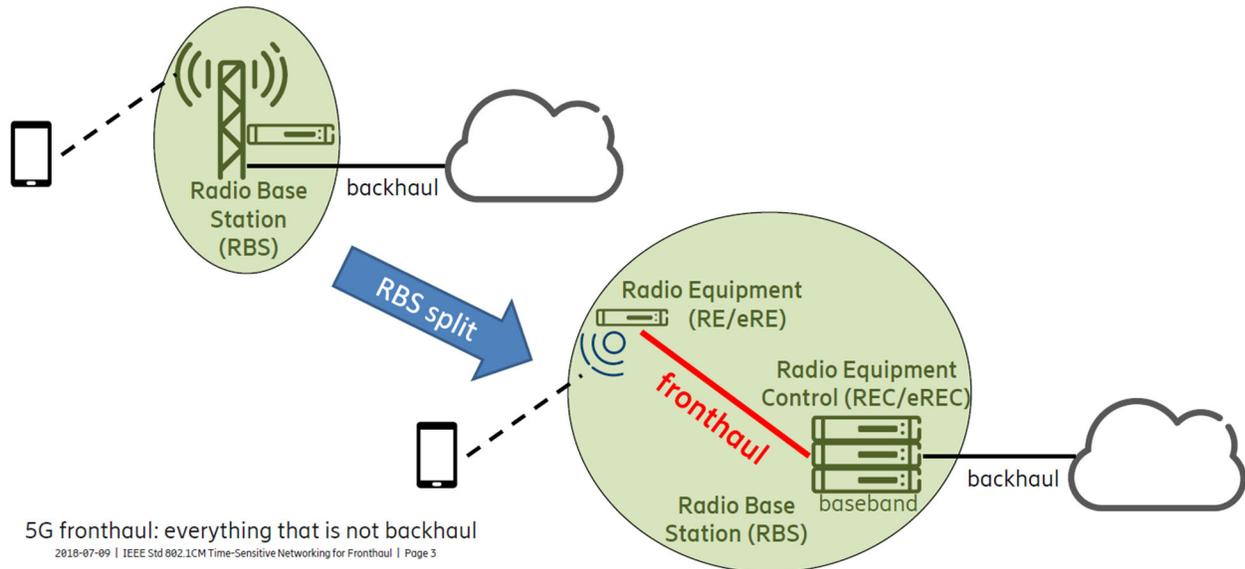
IEEE 802.1CM supports CPRI and eCPRI fronthaul interfaces via an Ethernet bridged network, thereby providing Ethernet-based fronthaul for both 4G and 5G. IEEE 802.1CM offers two solutions to meet the stringent requirements of fronthaul data flows. The mandatory base solution leverages the TSN toolset and aims for simplicity, a key driver in fronthaul networks, while the other solution leverages frame preemption as an additional tool if needed to achieve the required performance.
