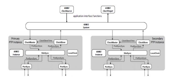
Figure 17-1—Model of hot standby redundancy for time synchronization
