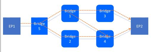
Flexible Positioning of CB functions. EP1 is not CB capable, EP2 is CB Capable
