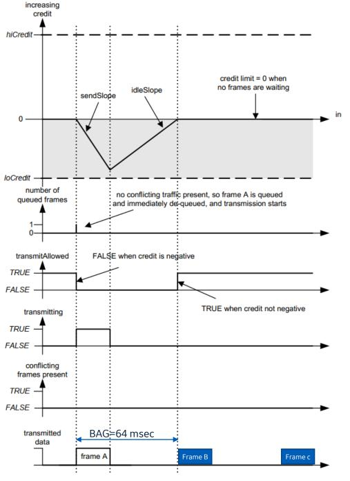
Figure L-1—Credit-based shaper operation—no conflicting traffic
