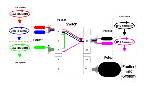
Traffic Shaping for Asynchronous Profile
