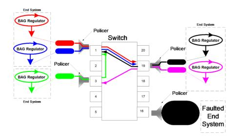
Example of VL1 with BAG of 64 milliseconds and VL2 with BAG of 128 milliseconds
