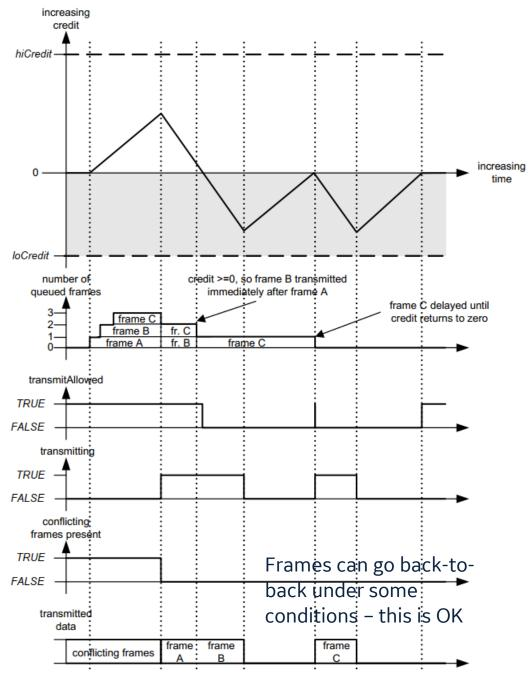
Figure L-3—Credit-based shaper operation—burst traffic
