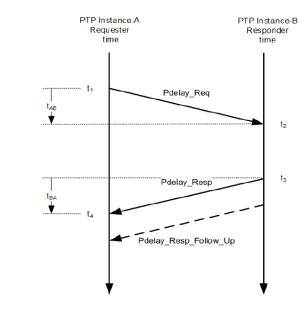
Figure 42—Peer-to-peer delay link measurement
