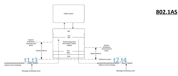
Figure 8-2—Definition of message timestamp point, reference plane, timestamp measurement plane, and latency constants
