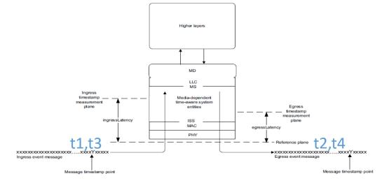
Figure 8-2—Definition of message timestamp point, reference plane, timestamp measurement plane, and latency constants
