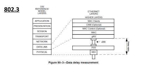
802.3 supports time sync by putting measurement timestamp point at xMII and providing PHY data delay(managed objects) as egress/ingress Latency.
